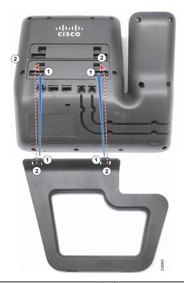
1 Insert the curved connectors into the lower slots.
